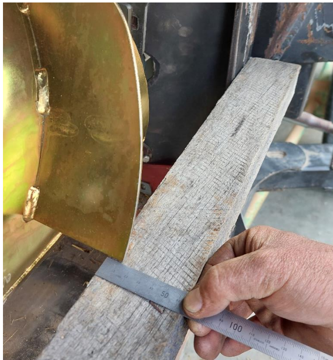
Figure 10: Typhoon flights excessively protruding past the adapter mount face.
