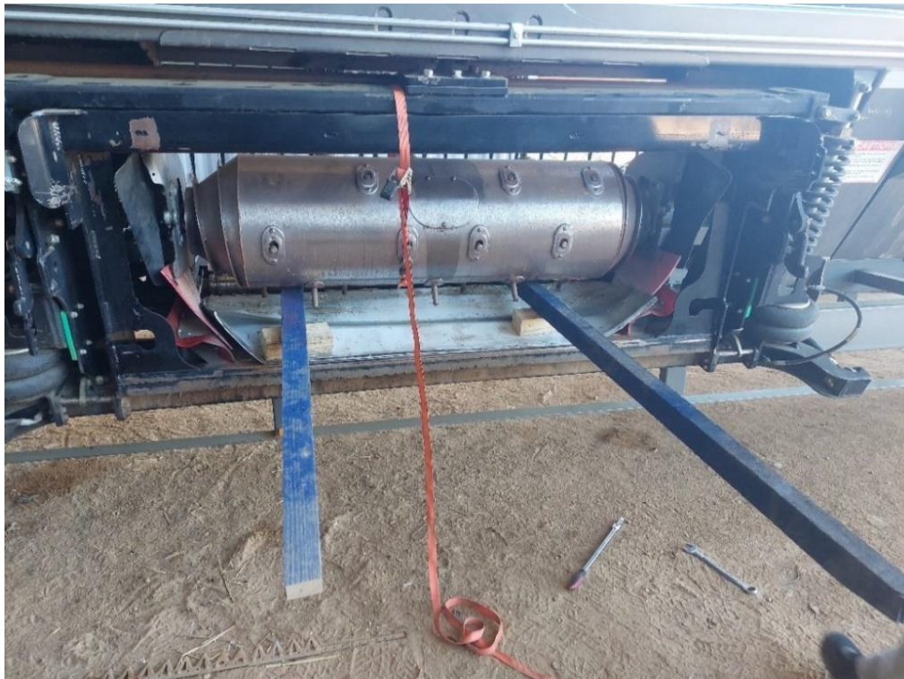
Figure 2: Securing the feed drum with a ratchet strap.
